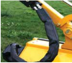
Bundle & protect hoses exposed to ultraviolet (UV) rays & abrasion.
