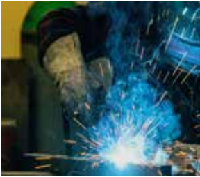
Protect weld cable from spark & spall.
