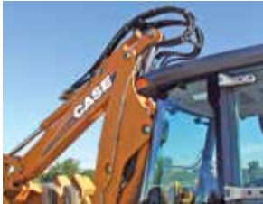
1050 remains tough & flexible in tight bend radius applications.
