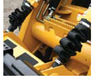
Hydraulic cylinders rely on the flexibility of 5601 to prevent contamination to piston rods.
