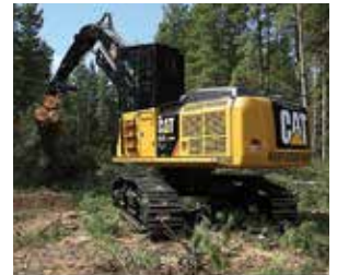
Forestry equipment utilizes 40 HDA where extreme abrasive conditions cause catastrophic hose failure.
