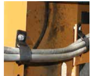
Hanging Straps provide a documented part location & allow access without the need for tools.
