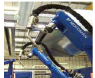
Weld Shield protects expensive hoses on large robotic welders.
