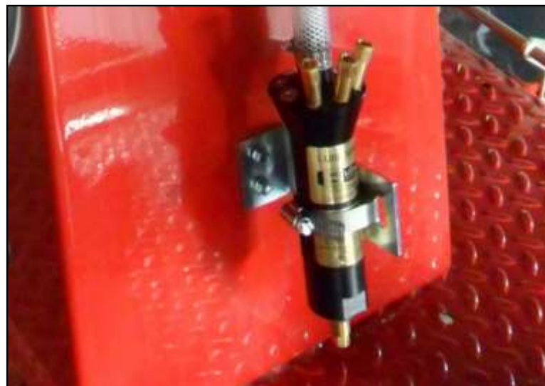
Step 3 Using pump bracket as a template, drill holes and mount bracket using 1/4" tap tight bolts. Secure pump to bracket with large hose clamp. Using the two small hose clamps, secure hose to pump and reservoir.
