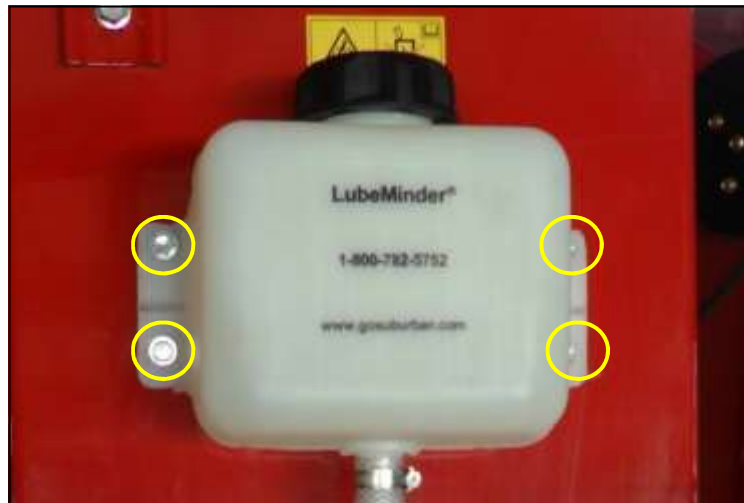
Step 2 Using the reservoir as a template, drill holes with provided drill bit. Secure mounting reservoir to shield using 1/4" tap tight bolts.
