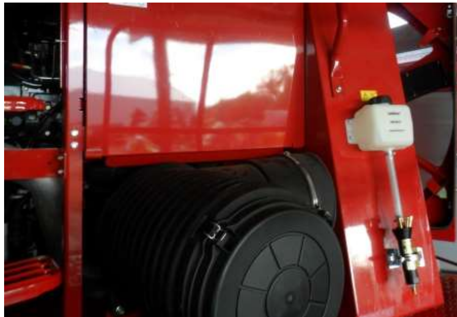
Step 1 Mock up Tank and Oiler mounting location. Make sure Oiler pump is at least 6 inches from the floor.
