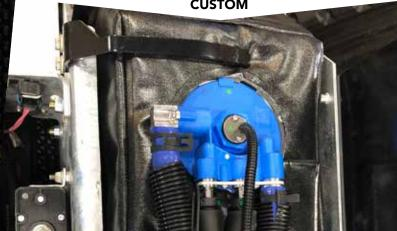
Concrete Pump Safety Cover: The concrete industry has recognized that safety is a must. The widely recognized Python Cover helps contain slurry and protect operators during pipe bursts.
