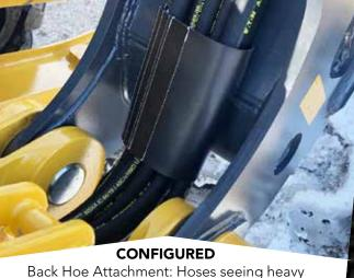
abrasion and pinch points are bundled and secured with internal grip straps.
